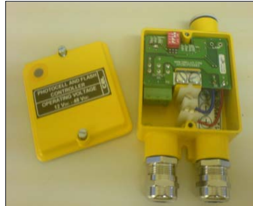
DC operated light unit with photocell & flasher
