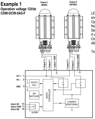
LED lights (LI-10-DCW-F) connected to both Output 1 (Main) and Output 2 (Spare).
