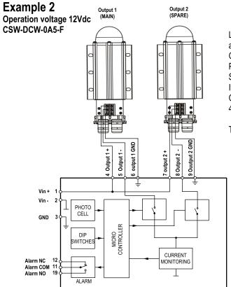
LED lights (LI-DCW-F) connected to both output 1 (Main) and output 2 (Spare).
